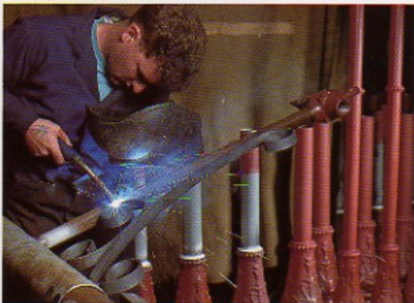
Welding a Scroll bracket.
