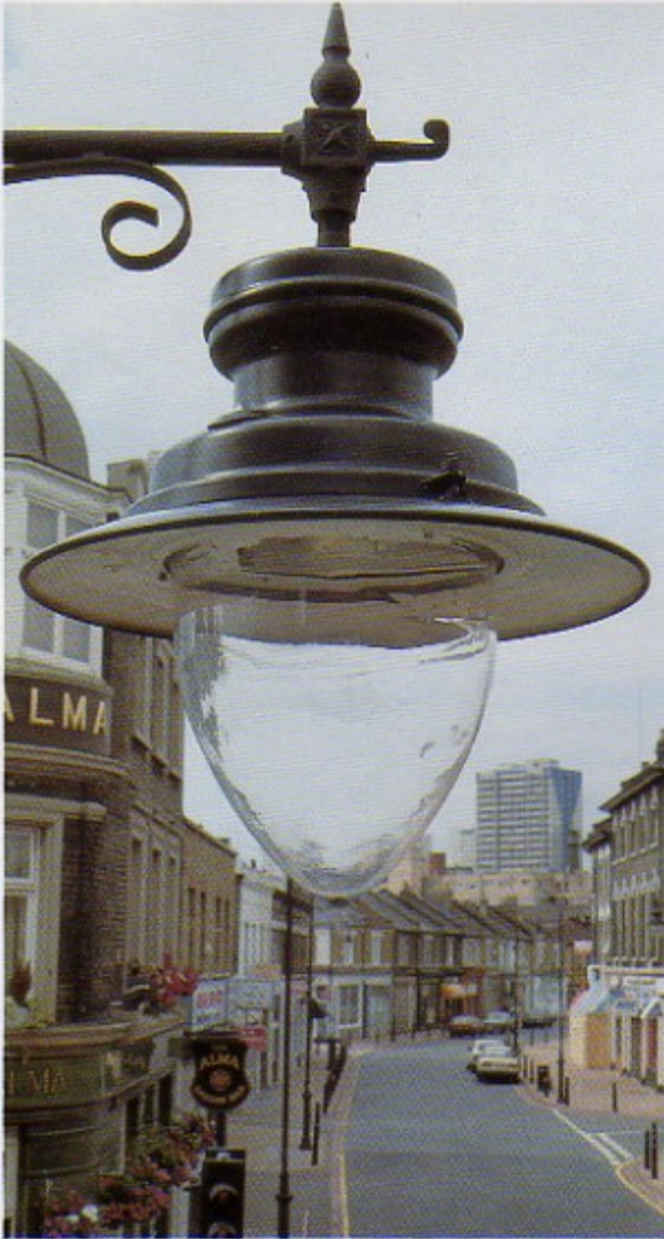
The reconstruction of Old York Road in the London Borough of Wandsworth included the installation of Strand B lanterns on Edinburgh columns.
