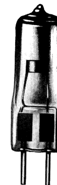
A1/216 Tungsten Halogen Lamp The A1/216 which operates on the Tungsten Halogen principle, has been designed primarily as a light source for 35 mm slide projectors. Although of only 150W rating, machines utilizing this lamp may achieve a screen illumination equal to that given by many projectors using a conventional mains voltage 500W Lamp.
