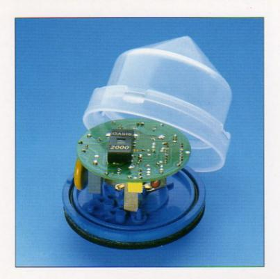
This new electronic photocell unit embodies state of the art technology. The integrated circuit contains a 'state machine' which eliminates cycling caused by transient light changes, and a silicon photodiode, filtered to closely match the CIE photopic curve. The combining of detection and switching circuitry on a single slab of silicon ensures extremely accurate night to night, and unit to unit switching, with no drift in switching levels.
