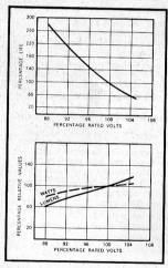
These curves are based on averages obtained with many lamps, and may be used as an approximate quide to performance. Theoretical values of extended life may not be realised in practice, since factors such as vibration, handling, cleaning and frequency of switching have an appreciable effect on lamp life.
