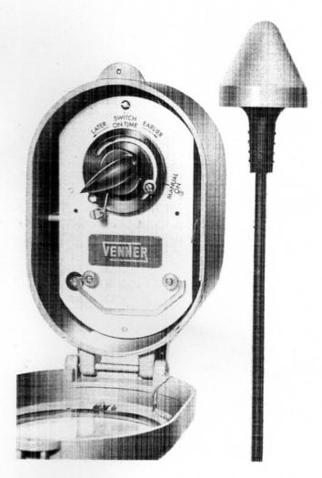
A delay of approximately 30 seconds prevents false switching due to transient cloud movement or spurious flashes of light. The photo-electric cell is housed in a translucent plastic housing, the plastic chosen being completely non-oxidising and impervious to discolouration from dirt and soot. The properties of the plastic also afford maximum protection for the cell, filtering out harmful ultra-violet rays.
