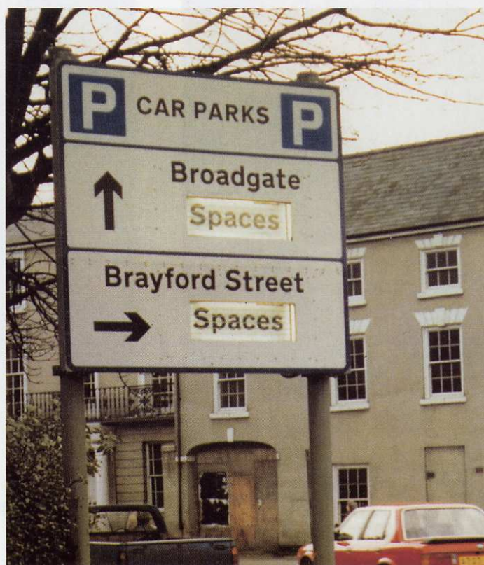
TWO EXAMPLES OF SIGNS WITH VARIABLE PANELS INTEGRALLY ILLUMINATED BY FLUORESCENT TUBES
