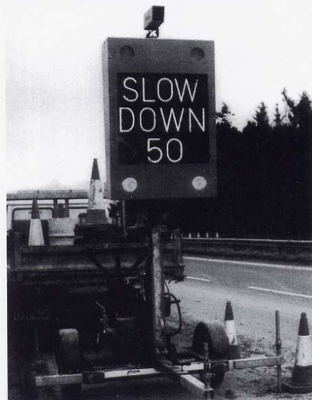
Trailer Mounted Speed Activated Sign
