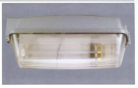
The Beta 5 is designed for use with a 35W SOX lamp and employs a pulse ignitor circuit for use on 240V 50Hz supply. For alternative voltages leaky field transformer gear is used.
