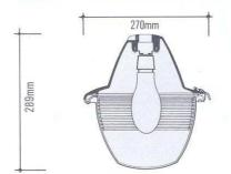
Maximum weight: 1.70 kg Windage area: 0.047m<sup>2</sup> Recommended mounting height: 5m Mounting: Top entry for 3 " BSP thread x 18mm
