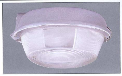
The Beta 7 is a minor road lighting luminaire of robust construction for use with a 70W high pressure sodium or 80 or 125W mercury lamp, and can be mounted on THORN 5m aluminium columns.
