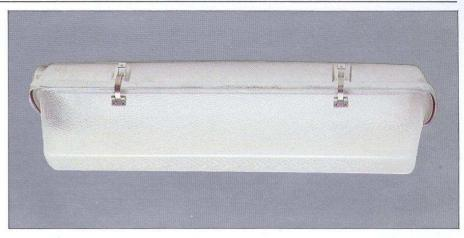
The Beta 6 for minor road lighting utilises two 40W 600mm long fluorescent tubes, and is complete with instant start integral control gear, all suitable for mounting on THORN 5m aluminium column reference QCO.
